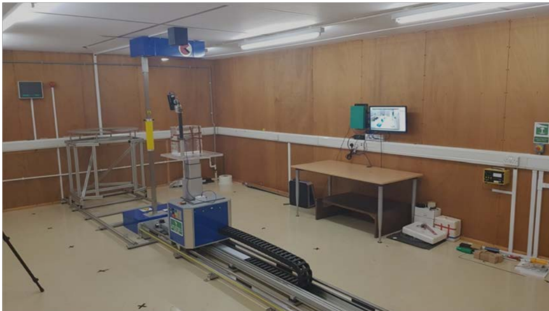
Figure 4: The PHE Neutron Laboratory in routine use. The ^{241}\text{Am-Be} source is contained within a steel tube, itself partially encased within a lead shield (painted yellow). A moveable platform allows objects to be placed at different distances (and heights) along a central axis away from the source.
