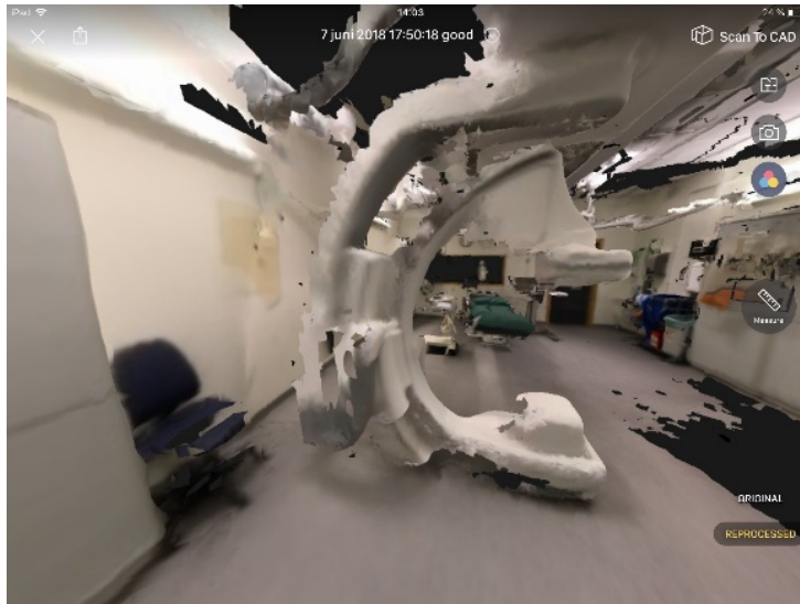
Figure 1. Print screen of the generated 3D mesh of the operating room using Structure sensors and the app Canvas.
